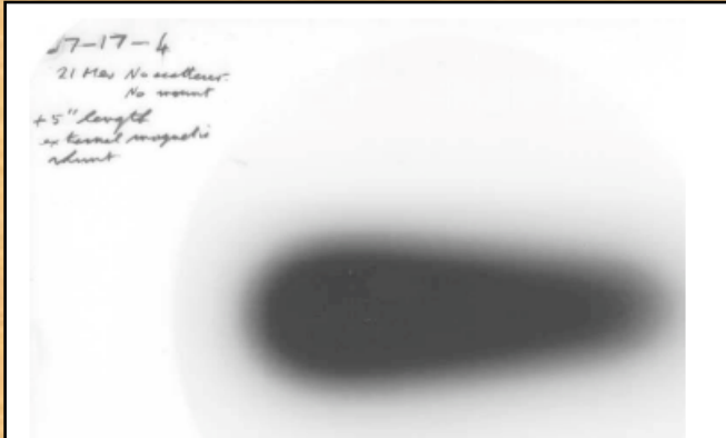
21 MeV 'natural' electron beam at open aperture in door, showing asymmetry caused by fringing magnet field; the problem was to achieve a uniform 'scattered' beam for use. 1961 developmental work; Kodak 'Translite' pearl-based film.
