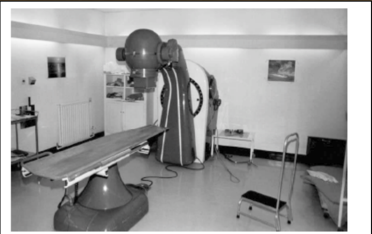
Palmerston North Hospital first supervoltage unit: Barazzetti Co-60, 55 cm SAD unit, installed 1958.
