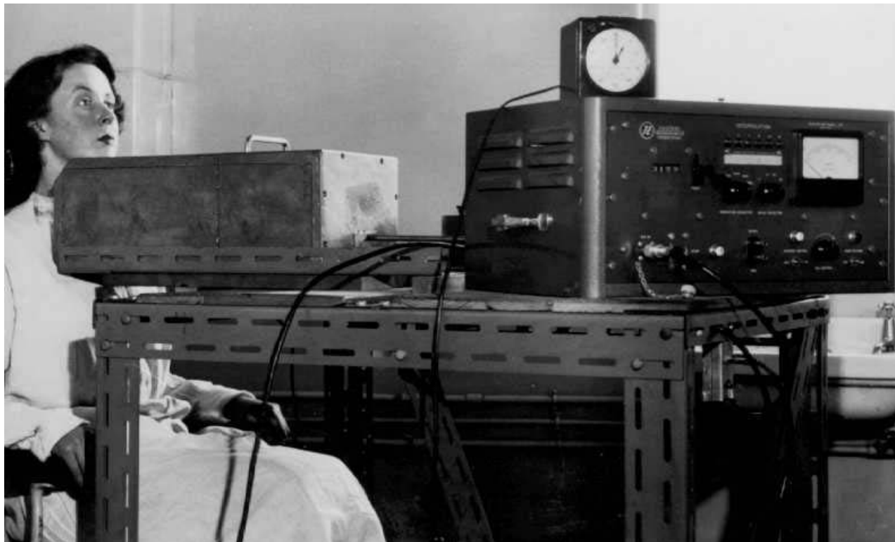
I-131 thyroid uptake equipment, 1952, as developed by Thyroid Research Unit, Otago Medical School. Two G26.Pb geiger tubes; 25 mm lead-walled 'castle'; perspex neckbar; good geometry, with 20 inches (50 cm) distance from geiger tube to neckbar; Note binary '64 Scaler' with separate timer. 'Patient' seated in dental chair for easy positioning. 15 uCi (550 kBq) given.
