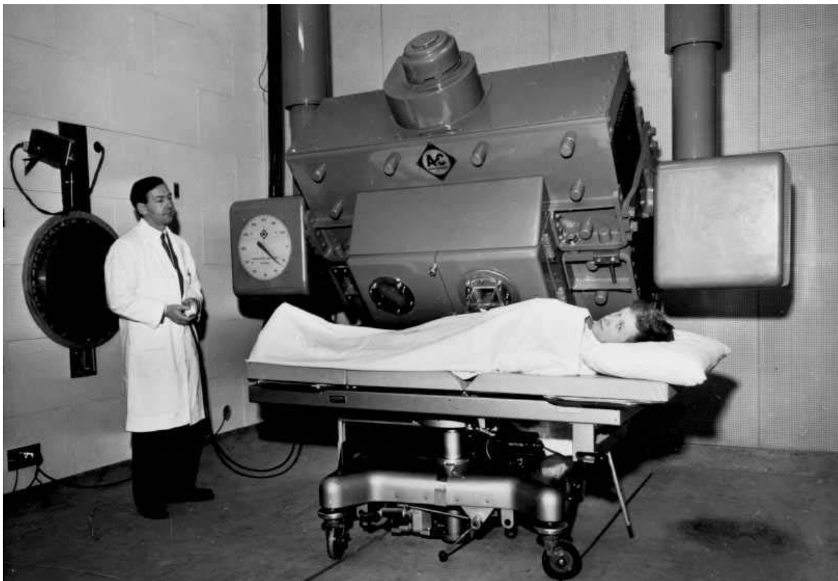
Allis-Chalmers 24 MeV Betatron, Wakari Hospital, March 1958 (Dr Frank Ramsay holding pendant controls; Howard Tripp as simulated patient. Note 60 cm dia water window; TV camera.
