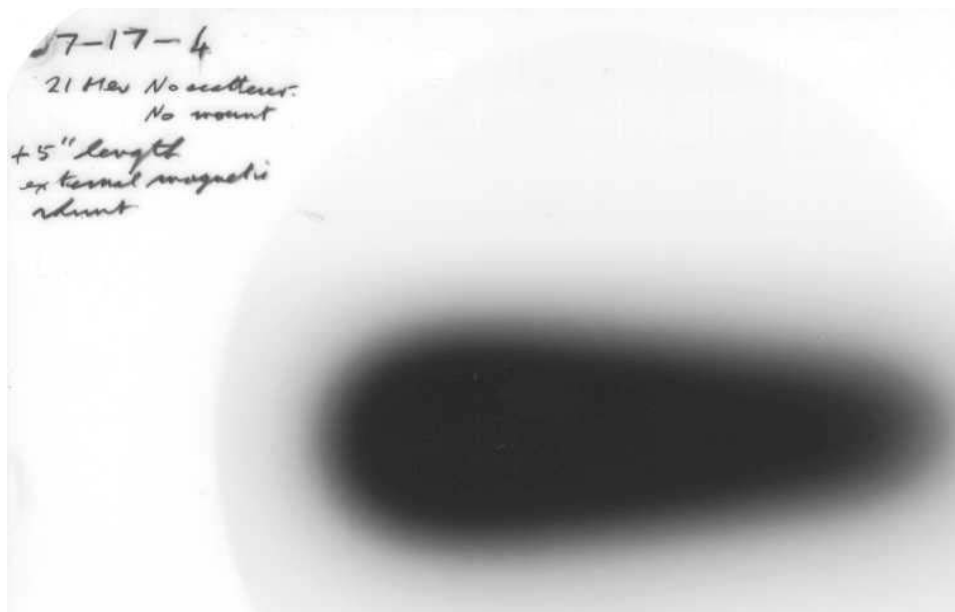
21 MeV 'natural' electron beam at open aperture in door, showing asymmetry caused by fringing magnet field; the problem was to achieve a uniform 'scattered' beam for use. 1961 developmental work; Kodak 'Translite' pearl-based film.
