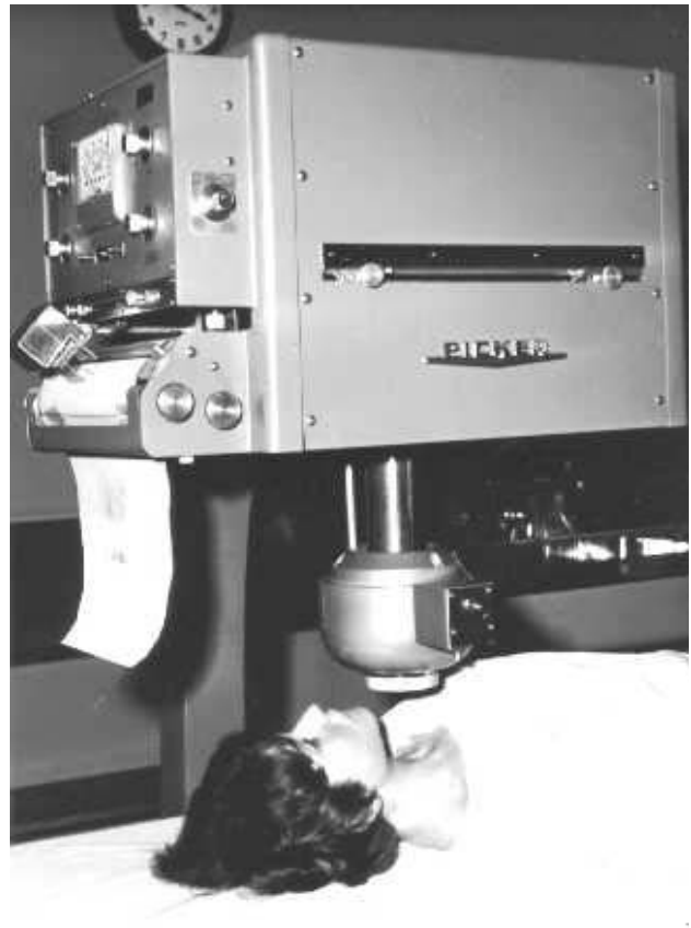
Modified Cliniscanner, with added colour printout; now ceiling-mounted over (former) X-ray table; 1967
