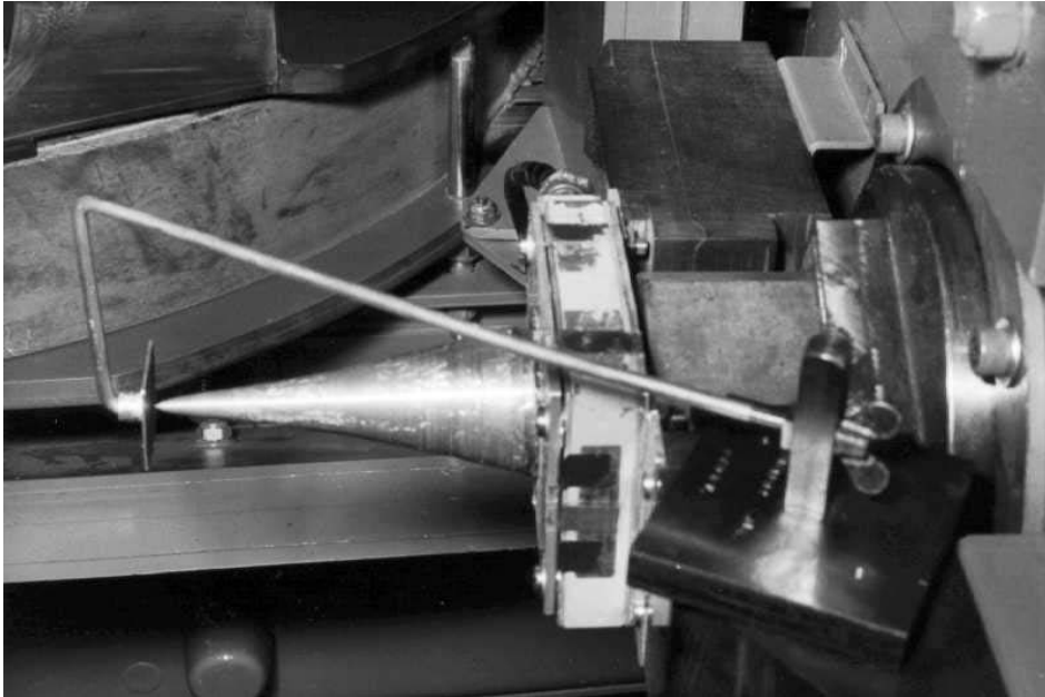
Betatron: Inside magnet doors, showing aluminium conical compensator, with our alignment jig in place. Also visible, magnet field coils, transmission monitor. 1958.
