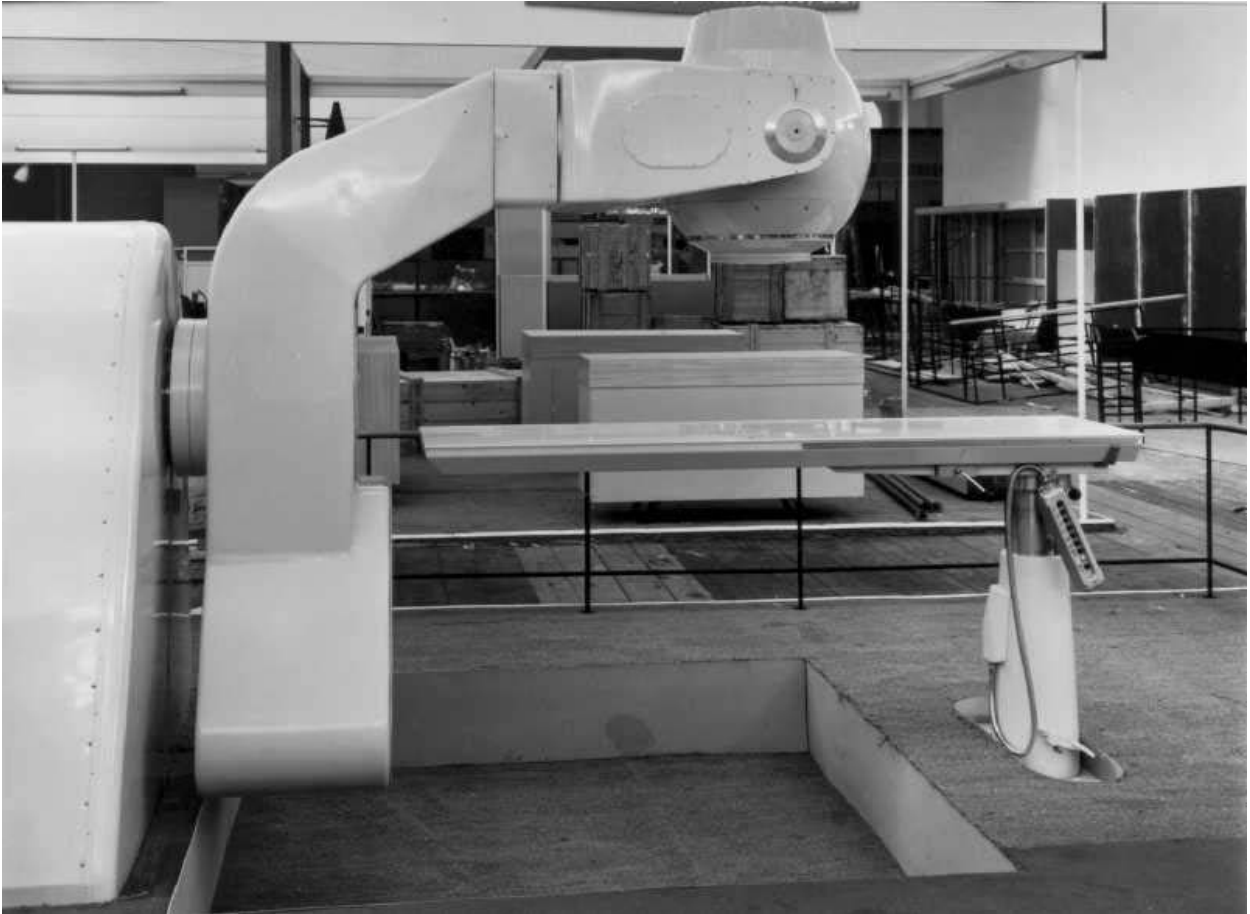
TEM Mobaltron, Co-60 unit, 75 cm SAD; similar to unit installed at Wellington Hospital, 1962
